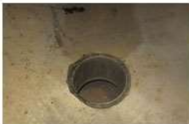
Figure 1. The inside of a pressure vessel nozzle that has been in service.
